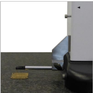
Height measurements on watch movement plate
