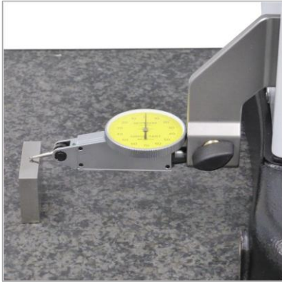
Fine adjustment for specific applications requiring an accurate carriage position
